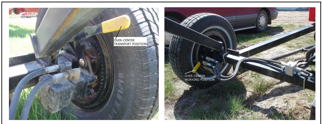
Figure 4.1 Over-Center Transport and Working Position
